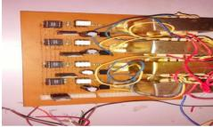
Fig8. Isolation and Driver Circuit.
